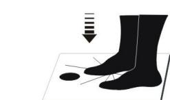
AUTO STEP ON – just step on the scale and stand still, the scale will automatically turn ON and start taking measurements.
