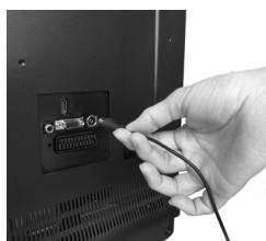
Connect the end of the coaxial cable to the TV's RF input socket.
