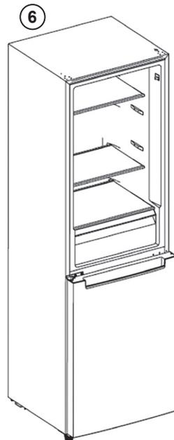
6. Take the fridge door, make sure the down hinge axis and the axis hole on the lower left side on the machine fix well and connect correctly; the fridge door is basically fixed now. Then use the screws which were taken down in the step one, to fix the upper hinge on the left side of the cabinet; then put on the upper hinge cover, then fix it by the screws.
